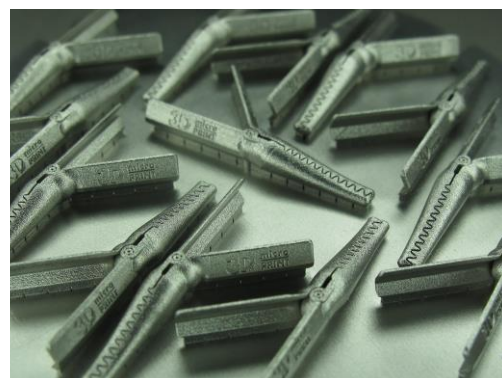
Figure 5: Several grabbers on a building platform
